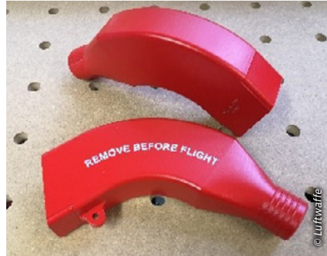
3D-printed hose-to-nozzle connector for the Eurofighter. The printed material is suitable for use with the relevant fluids (Antero material).
